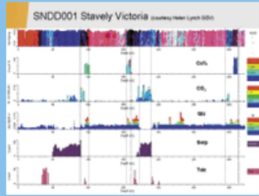
*This figure, from the Stavelly region in western Victoria and courtesy of Helen Lynch at Geoscience Victoria, shows a combination of logs from a variety of wavelengths. The thermal infrared in particular is mapping smaller proportions of carbonates than previously possible, as well as highlighting a number of quartz vein systems.*
