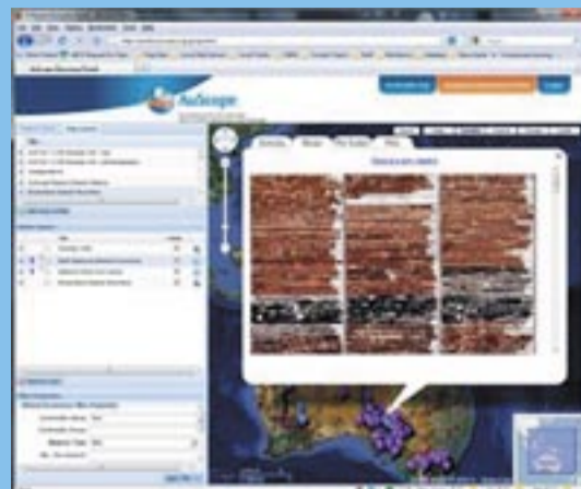
v2.3 of the AuScope Portal displaying NVCL boreholes and a mosaic of a selected borehole's core tray. Additionally, occurrences of Iron in Australia and Earth Imaging seismic recorder locations are displayed.
