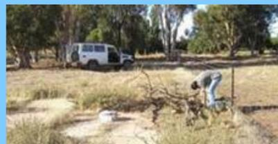
Passive seismic collection.
