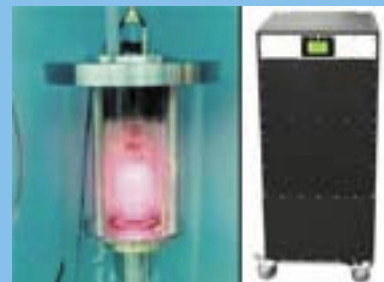
A hydrogen radio frequency discharge, the first element inside a hydrogen maser.
