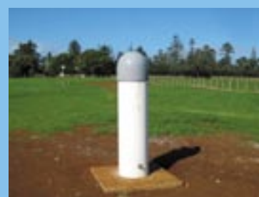
Typical AuScope GNSS installation at Norfolk Island.
