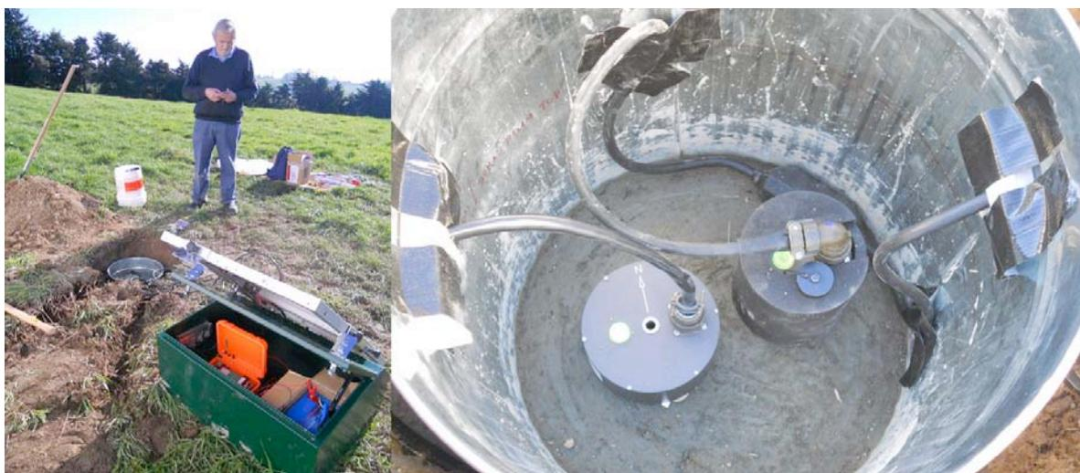
***Left: Deployment of aftershock seismometers in Gippsland. Right: Close-up view of aftershock seismometer in place in Gippsland.***
