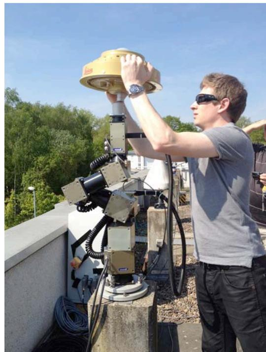
***GNSS Robotic Calibration System***
