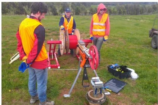
The borehole thermal logging and in-situ thermal conductivity logging capability is now in place with the receipt of an AP-Sensing GeoDTS system including several lengths of active and passive optic fibre sensors. A new deployment system has been developed and the equipment has been successfully tested in the field at Tynong.
