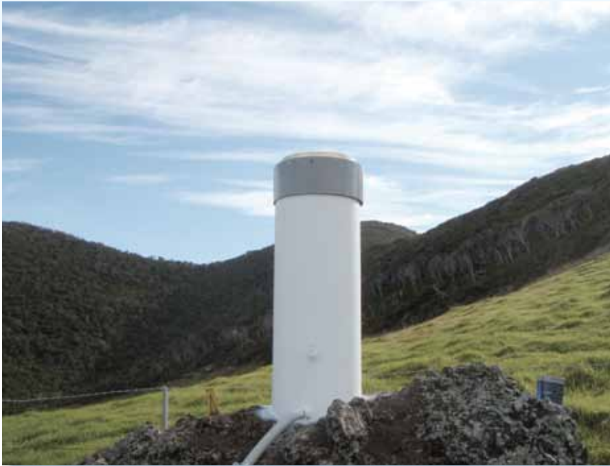
The GNSS site at Lord Howe Island is one of the stations being built across Australia.
