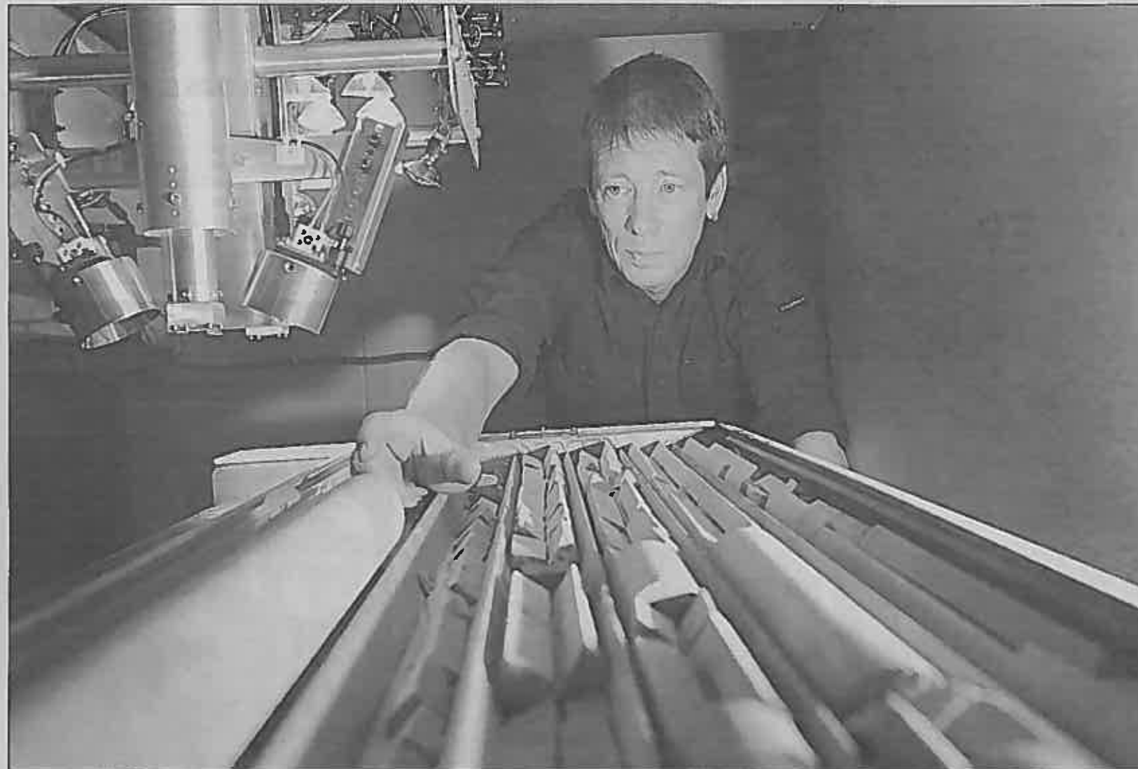
HyLogger operator Darren Bowbridge examines core samples as part of an NT Government program to encourage companies to explore for minerals in the Northern Territory
